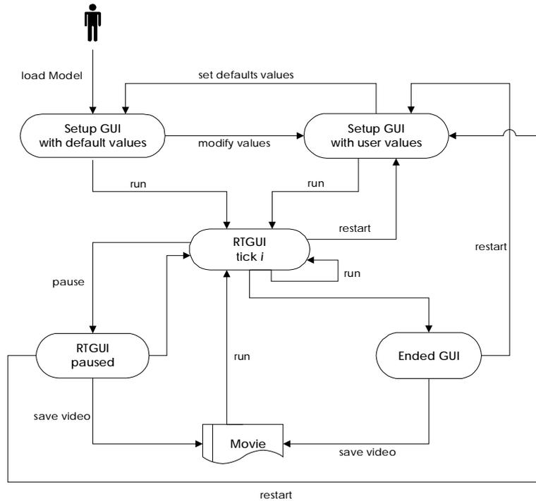
First, as we saw before, the model is loaded and Simma shows the Setup GUI with the default values set by the model. At this moment the user can start the simulation with these values or change them.
